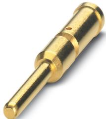
Crimp contact, turned, contact diameter: 2 mm, crimp range: 0.25 mm<sup>2</sup> ... 1 mm<sup>2</sup>
